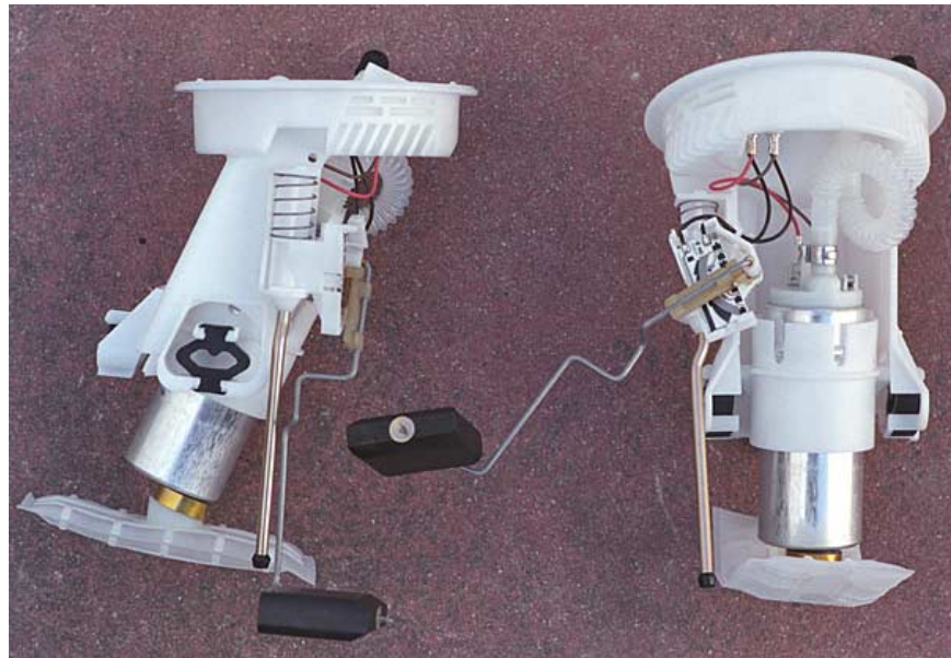
Figure 3: Fuel Pump Assembly: BMW P/N 16 14 1 182 842
