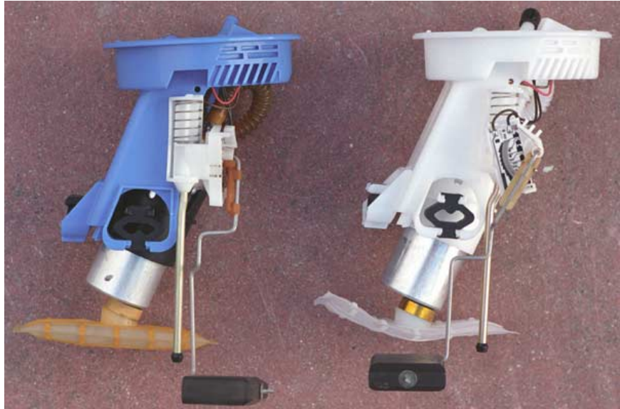
Figure 12: Comparison of Stock and Modified Pump Assemblies
