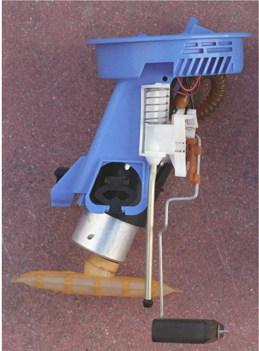
Figure 8: Stock Fuel Pump with Sender, Side View
