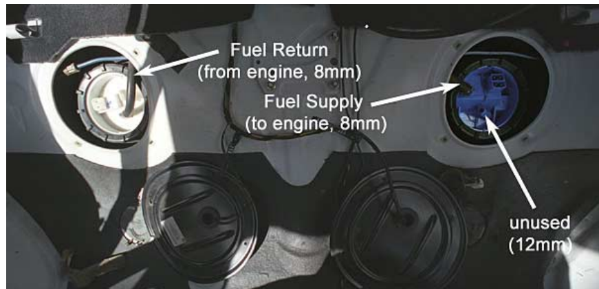
Figure 6: Stock Fuel Supply and Return Layout (1/95 and later)
