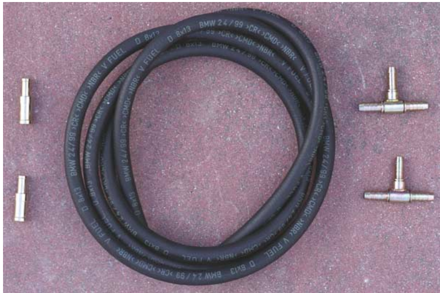
Figure 4: 8mm Fuel Hose, Adapters and Ts
