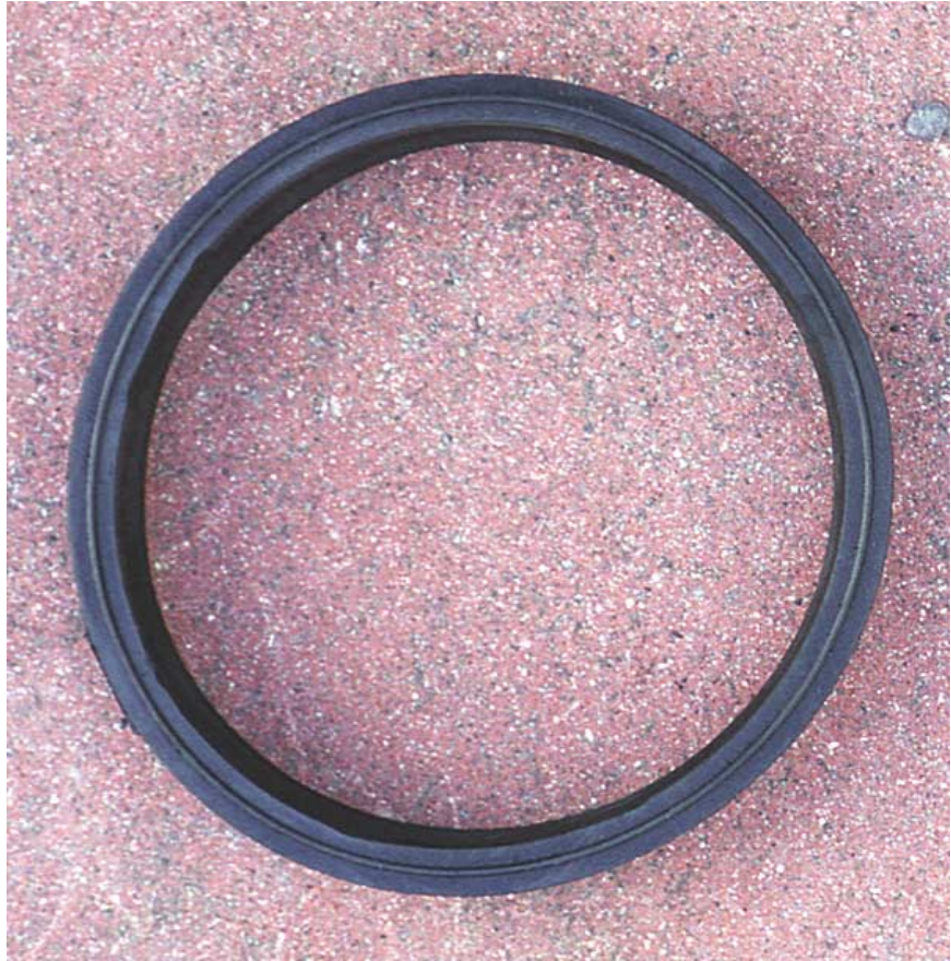
Figure 9: Fuel Pump Seal (Top View)
